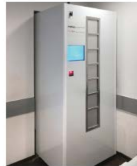
Software and barcode-scans guide pharmacy staff to the next available location for order storage
